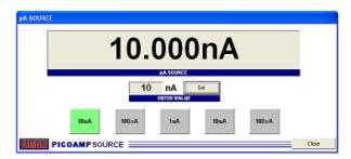
Connect Picoamp source and select range required by using the range selection buttons
